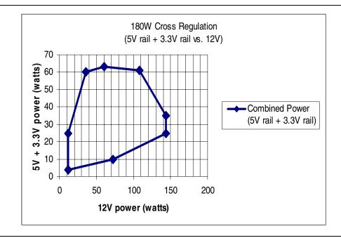
Figure 2. Cross Loading Graph for 180W Configuration
